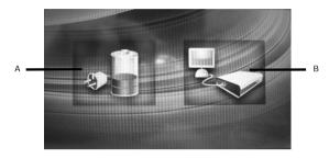
When the navigator is connected to computer using USB cable, the screen above will appear. Tap  $\bf{A}$  to only charge the battery of the navigator and  $\bf{B}$  to access to the navigator's storage (for file transfer).
