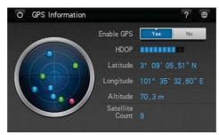
Screen will display the position of GPS satellites, latitude, longitude, altitude, satellite count and HDOP bars.
