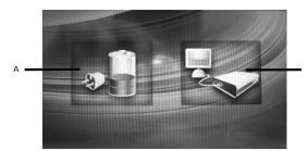
When the navigator is connected to computer using USB cable, the screen above will appear. Tap **A** to only charge the battery of the navigator and **B** to access to the navigator's storage (for file transfer).
