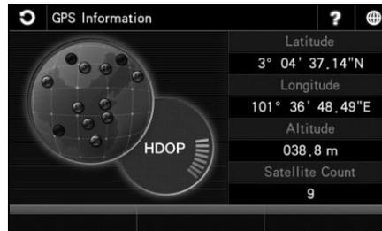
3. Screen will display the position of GPS satellites, latitude, longitude, altitude, satellite count and HDOP bars.
